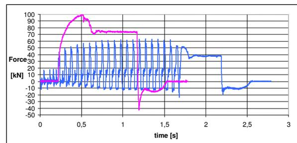
Due to small forming steps the axial forces are reduced by 40 %
